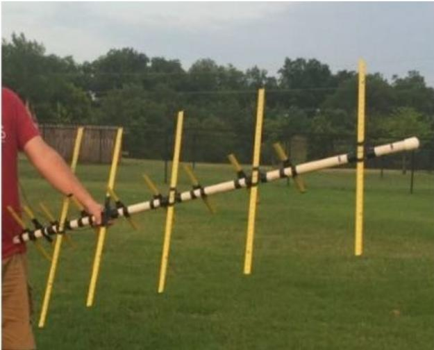
The element holders are attached to the boom with electrical tape in the photo above. While I haven't tried it, I'd suggest that the antenna might be a bit more robust if you could screw or perhaps glue the holders to the boom.
