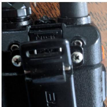
Looking at the back there are four screws ignore the two that are for the belt clip - the other two are torque screws and used to hold the case together.
